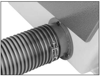
**Figure 26.** Flexible dust hose connected to dust port.
